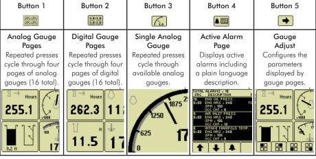
Note: Most problems with electronically controlled engines can be pinpointed via ECU diagnostic messages.
