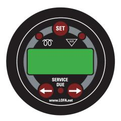
The DPG features a backlit LCD display with three push buttons in a 2" gauge. Additionally, three bright LEDs indicate Preheat, Service Due and Auxiliary input. The LCD is clearly readable in both bright sunlight as well as total darkness. The DPG allows each system to be field configured to suit the customer's unique requirements. After initial configuration, the DPG can be removed in cost sensitive applications.
